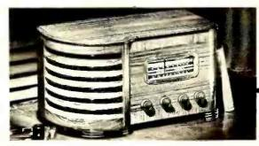
6 TUBE MOOEL 0-12. A two-band AC-DC Superhet of brilliant styling. Tunes 1720 to 535 K.C.; 2200 to 7000 K.C. Features: 2 Watts Output; Beam Power Tube; Tone Control; A.V.C.; 6" Slide Rule Olal; 6" Electro-dynamic Speaker. Size: 16"X71/2"x994". The new type table cabinet has the exclusive SONORA louvre grille.
